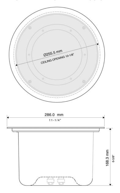
Rough opening without preconstruction bracket is 10.25 inches in diameter
