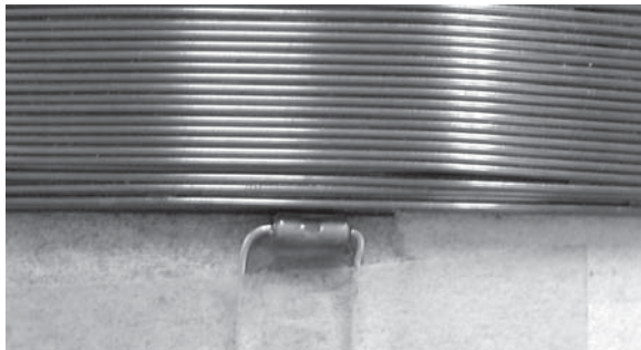
Heat sensor on voice coil
