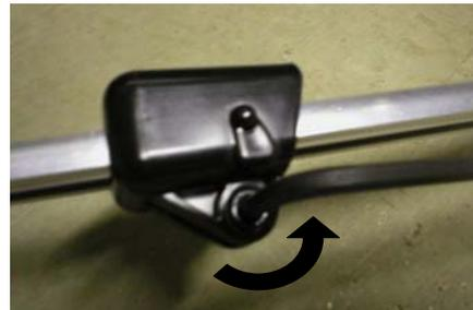
**NOTE:** Heavy corrosion inside load bar could prevent smooth operation. Clean as necessary.
