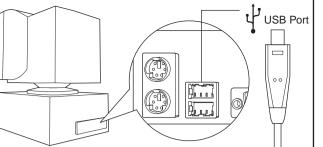
Connect the other end of the USB cable into the USB port on your computer.
