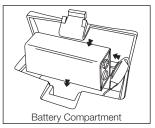
**Note:** You should replace the battery every six months, or after any extended power outage that could drain the battery power.
