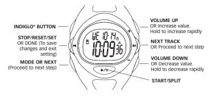
When setting, each button has a different function as indicated above. Display indicates when button changes function.
