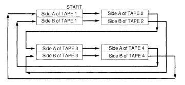
(b) When the sequence selection switch of both units is set to A-B-A-B position ( $\supset$ ).
