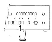
Depress the REC RUN button. The RUN LED illuminates (the SPACE LED also illuminates) and the tape begins to travel to permit recording.
