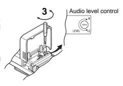
**Step 4.** Adjust the corresponding tuner's volume control so that its knob points to the 2 o'clock position. If the tuner's AF PEAK indicator remains lit, readjust the microphone's audio level control to the position that causes the indicator to flash when the tuner output level reaches its peak. The AF PEAK indicator lights when the output level reaches the point of about 3 dB below the clipping level.
