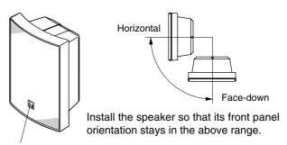
Install with the logo mark located at the bottom of the front panel.
