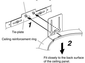
If the ceiling reinforcement ring does not line up accurately with the ceiling mounting hole, adjust its position by either loosening the tieplate mounting screws and sliding the tieplate into correct position, or by shifting the tie-plate mounting screws to the appropriate holes in the Tile Bridge rails.
