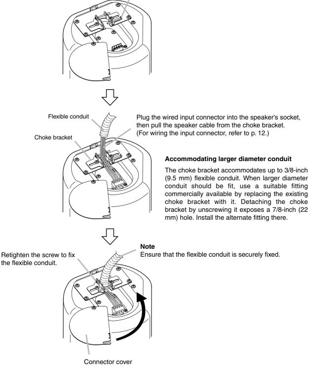
After completing the speaker cable connection, turn the connector cover in the direction indicated by the arrow, and fix the cover with 2 screws.
