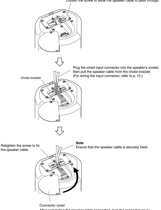
Loosen the screw to allow the speaker cable to pass through.
