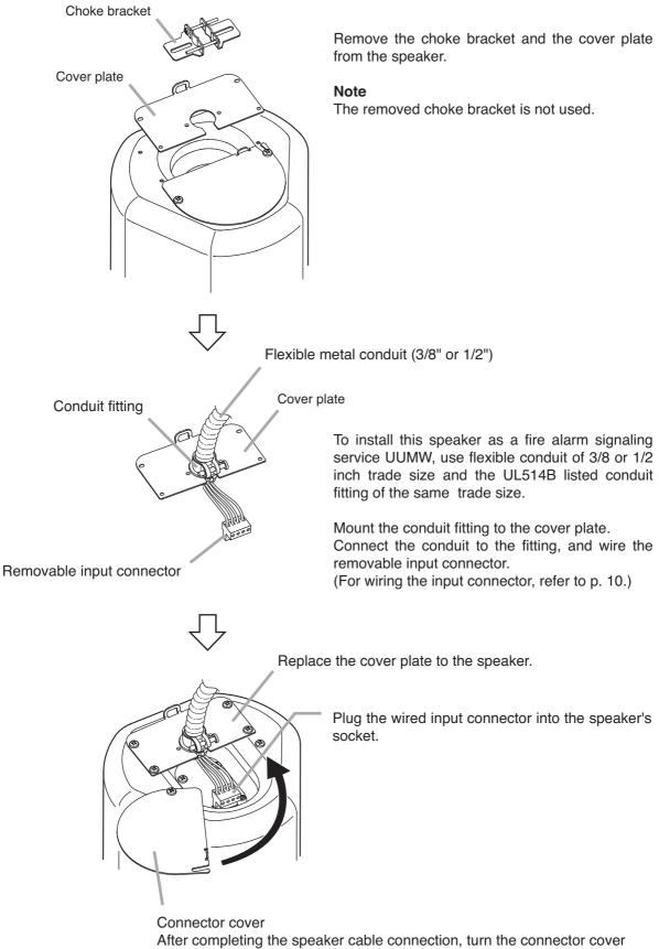
After completing the speaker cable connection, turn the connector cove in the direction indicated by the arrow, and fix the cover with 2 screws.
