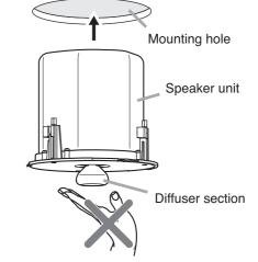
Rotate and tighten the mounting tab axis screws (3 places) on the unit clockwise to their full stop in order to grip the ceiling panel with the mounting tabs.
