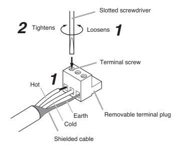
**Tip**Recommended slotted screwdriver type: Screwdriver with blade that is 3 mm in width
