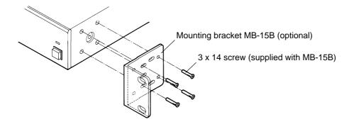
Step 3. Using other screws also supplied with the MB-15B, mount the unit in the rack.
