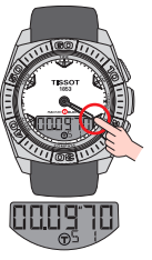
Touch twice to access saved split times
