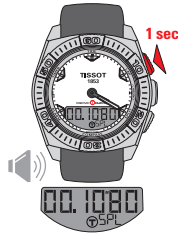
Last arrival time must be stopped with the + pusher
