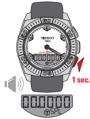
Reset split chronograph with the - pusher Arrival times are saved as long as the split chronograph is not started again
