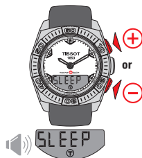
b) + / - : stop the count, the watch does not switch to standby mode
