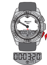
Reload the last time set on the timer
