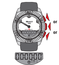
Stop the ringing with any pusher
