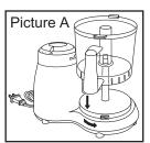
Place the Discharge Disc onto the Drive Shaft. (See Picture B)
