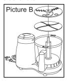
Place the Slicing/Shredding Disc on the Drive Shaft. (See Above Picture B)
