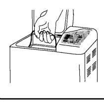
Mount the kneading blade on the shaft, flat side down.
