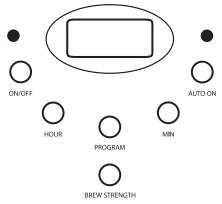
**Power ON/OFF Button:** Use this button to turn the unit on and start the brewing process. You can also turn the unit off by pressing this button when the brewing cycle is complete.
