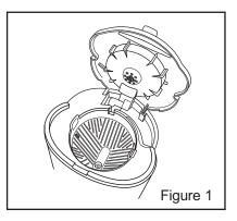
**Note:** The Removable Filter Basket must be placed into the coffeemaker with the two handles, located on the sides of the Filter Basket, aligning with the two notches on the inside of the unit (see Figure 1 on previous page). Press the Filter Basket down until it clicks into place.
