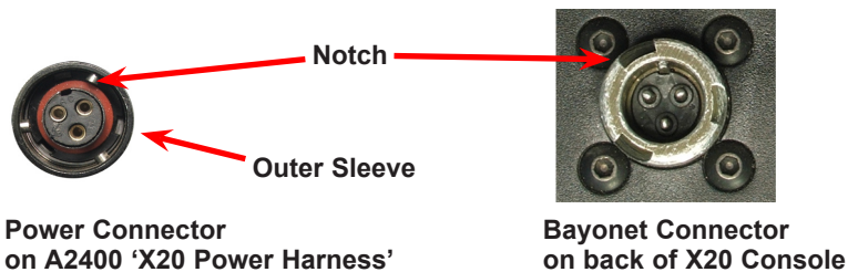
Figure 4-3. Connecting the Power Connector
