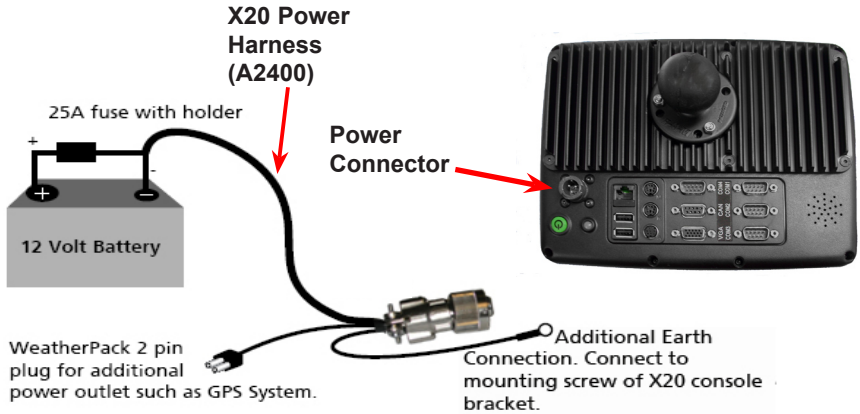
Figure 4-2. Layout of the X20 Power Harness
