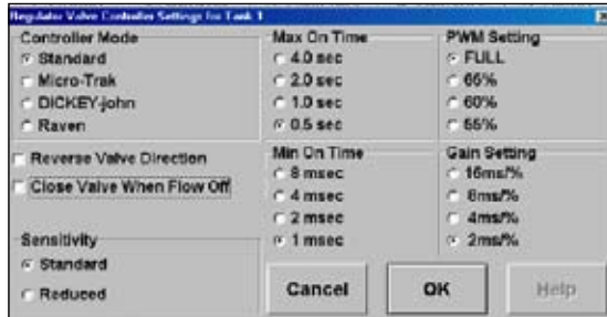
Figure 8-5. Regulator Valve Settings
