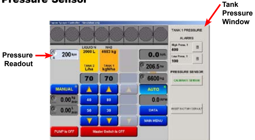
Figure 10-1. Working Screen Showing Tank Pressure Window
