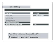
Press the button to move and adjust the motor to a certain position of the East limit. Save it by pressing **red** (**F1**) button. The indicated number will be set as 1000.
