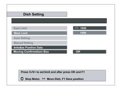
Press the button to move and adjust the motor to a certain position of the West limit. Save it by pressing **red** (F1) button.
