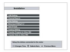
First, go to the Motorized Dish Setting under the Installation-Dish Setting-Auto Setting menu. Please note that the button always indicates the eastern direction and similarly the button always the western direction.
