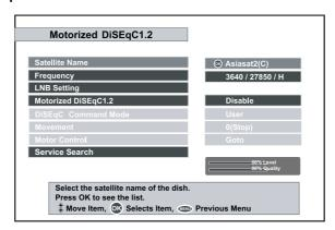
If you have DiSEqC 1.2 motorized system, then you can use the DiSEqC 1.2 functions.
