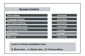
The Access Control menu controls access to following items: Time Setting, Language Setting, A/V Output Setting, Organizing Services, Organizing Favorites, Installation and IRD Lock. Press , buttons to Locked/Unlocked the access. Locked means controlling the access to the specific menus with the PIN Code system. The default PIN Code is 0000.
