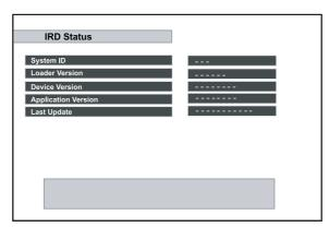
Check the STB's system information here. It shows the System ID, Loader Version, Device Version, Application Version and Last Update.
