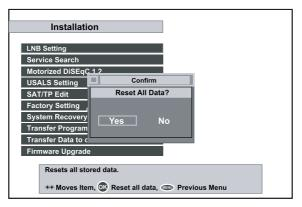
All the stored data can be reset just like it was manufactured. The factory setting has two steps. The first is to reset the service data and other system configurations except
