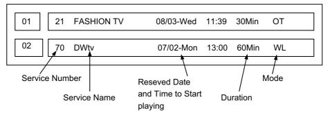
To insert new entry of Timer Setting, press (Red) Button. Press button to edit the entry, and press (Green) button to delete the selected entry.
