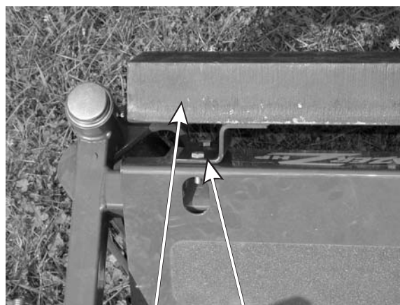
Figure 14 Front Weight Assembly
