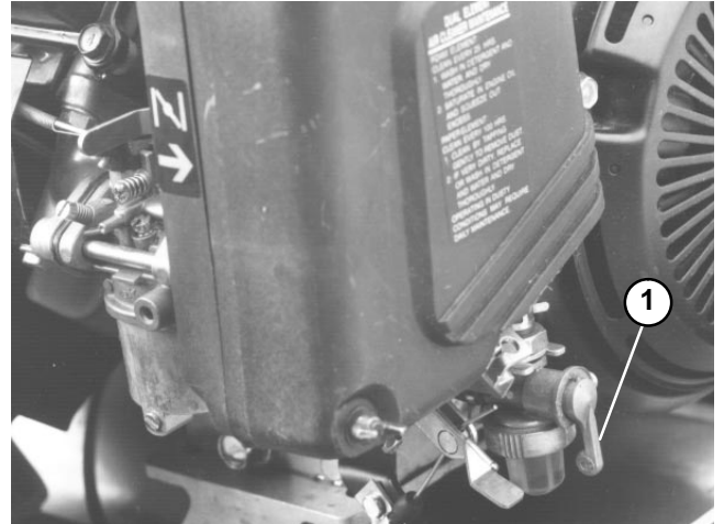
Figure 2 1. Fuel shut-off valve
