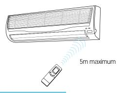
• You can hear a beeping sound from the unit in the following cases, which indicates that the signal is received.
