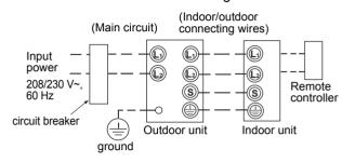
Connect the indoor/outdoor connecting wires to the identical terminal numbers on the terminal block of each unit.
