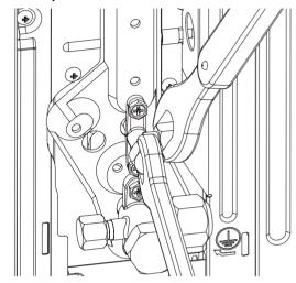
Use two wrenches to loosen or tighten the flare nut on the gas service valve as shown in the figure. Use only one wrench to loosen or tighten the flare not on the liquid service valve.
