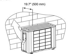
Install the unit so that the discharge is at a right angle relative to the wind direction.
