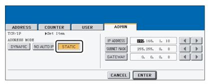
Press the [IP ADDRESS] button and enter the IP address of this device using the digital keys. Enter also the subnet mask and default gateway as required.
