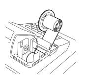
If the printer is used for Journal, hold down the **[FEED]** key to wind up the printed portion of paper, then cut the paper as shown in the figure. Hold down the **[FEED]** key again to advance the remaining paper end.
