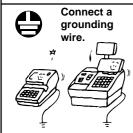
■ Ensure that the equipment is properly grounded. Extension cables should also be grounded. Fire or electric shock can occur on improperly grounded equipment.
