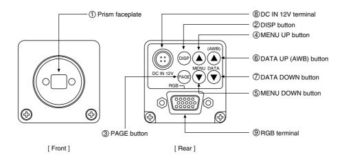
① Prism faceplate The protection cap is attached on the lens mount portion. After removing the cap, mount the lens. Be careful not to scratch or touch the optical area.
