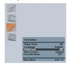
When Child Lock is selected, a reminder will appear when any of the top buttons are pressed. Once the television has been switched off it can ONLY be brought out of standby using the remote control.
