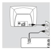
After everything is connected properly, plug in the AC power cord to the power outlet. Never make or change any connections with the power switched on.
