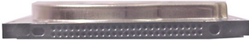
Figure 1. MK6006GAH HDD - INTERFACE CONNECTOR
