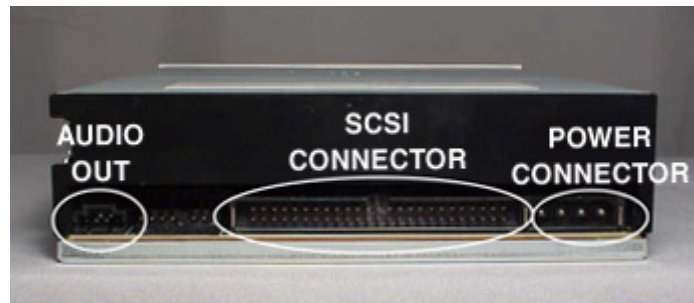
Figure 1. SD-M1711 DVD-ROM Drive Rear Panel - Connectors
