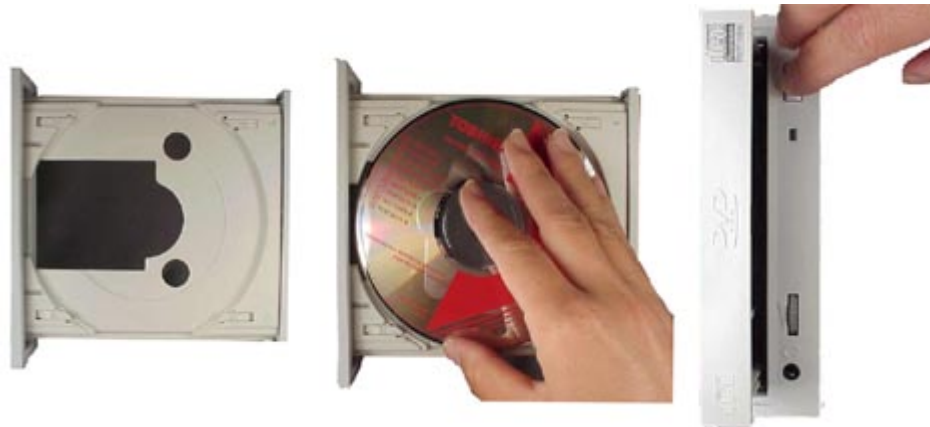
Figure 2. Inserting Disc Vertically
