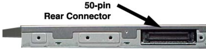
Figure 1. SD-R2312 DVD Writeable Drive Rear Panel – Connector
