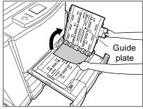
Push the lever to lift the lower guide plate. Make sure that the guide plate is latched to prevent it from dropping.
