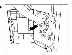
**3** Pull out the grip of the saddle stitch holder (①) toward you and turn it (②) 90° clockwise in the direction of the arrow.
