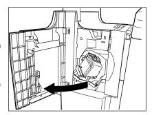
Turn the blue lever 90 degrees to the left and pull out the stapler unit.
