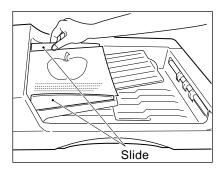
For setting large-size paper such as A3 or B4, pull out the paper folder in the direction of the arrow.
