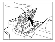
Lift knob ① or knobs ① and ②, then remove any misfed paper.
