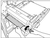
10 If the misfed paper cannot be removed in step 9, raise the exit guide of the fuser unit and remove it.
