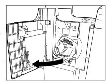
Turn the blue lever 90 degrees to the left and pull out the stapler unit.
