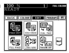
Press the LEFT (or RIGHT ) key according to your desired binding side.
