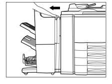
2 Open the cover of the hole punch unit.
