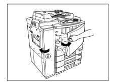
Remove the used toner bag from the copier in the direction of the arrow.
