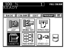
Press the drawer key corresponding to that in which the paper size has been changed.
