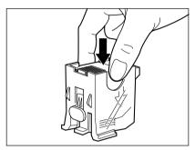
Pull out the seal which holds the staples horizontally.
