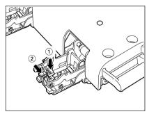
Remove any jammed staples, and then return the knob ② to its original position.
