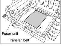
**9** If the misfed paper is gripped between the rollers, remove it by rotating the lever in the direction shown.
