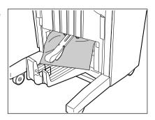
Open the exit cover of the saddle stitcher and remove any misfed paper.
