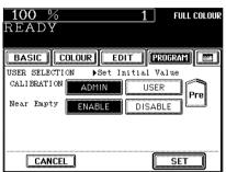
To change the initial settings of the automatic calibration and display of "Near Empty", you need to key in the administrator password (5 digits).
