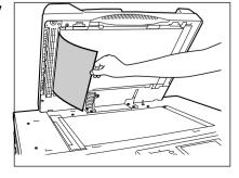
**3** Open the exit-side cover and remove any misfed originals.
