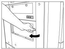
Put down the lower guide of the exit side and remove any misfed paper.
