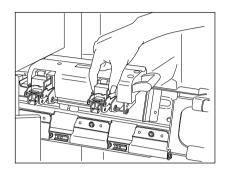
While pushing down on the lever  $^{\textcircled{1}}$ , pull up the knob  $^{\textcircled{2}}$ .
