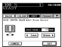
Utilizing this feature allows the facing pages of a book or magazine to be copied page by page onto two separate sheets of paper or duplex-copied on one sheet. There is no need to move the original on the glass. You can also place a pair of A4 (B5 or LT) sized originals side by side and copy them on separate sheets of paper.
