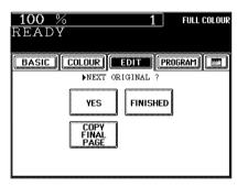
When the image occupies the entire original (to the edges), use Full Image Copying to reduce the ratio a little bit so that the edges of the image will not be missed.
