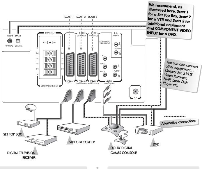
On the back of the TV are 3 Scart sockets, and a selection of phono sockets, all of which will enable you to connect a variety of equipment.
