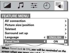
screen when you press any of the front panel buttons. Once the set has been switched off it can ONLY be brought out of standby using the remote control.
