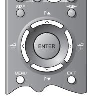
Most video recorders and Set Top Box receivers send a signal through the Scart lead to switch the TV to the correct *Input* socket. Alternatively you may select it with the external source selection button - on the remote control. Press - repeatedly until you see the picture on your equipment.
