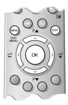
If you cannot connect your television to the video recorder using Scart leads you will need to allocate a programme position on the television for the video recorder. Insert a pre-recorded tape and press PLAY on the remote control, then Manual tune...
