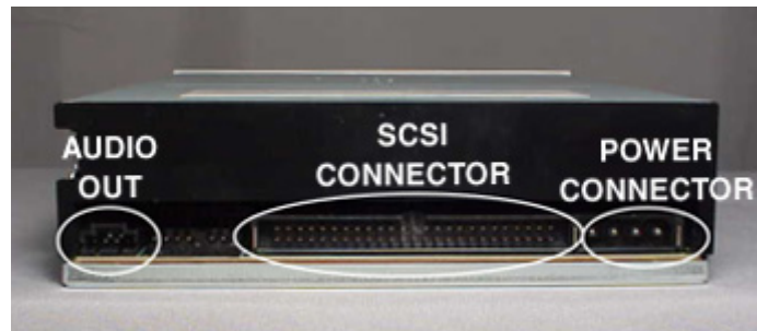
Figure 1. SD-M1401 DVD-ROM Drive Rear Panel - Connectors
