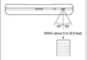
Distance: About 3 m (9.9 feet) from the front of the remote sensor
