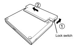
5 Attach the connector cover on the bottom of the player.
