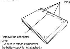
4 Turn the battery pack over and insert four catches into the player's corresponding holes. Then, slide the battery pack in the direction of the arrow ② until a "click" is heard.
