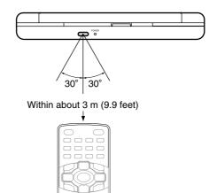
Distance: About 3 m (9.9 feet) from the front of the remote sensor
