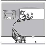
Use the composite video cable (yellow) to connect the DVD player's VIDEO(CVBS) jack to the video input jack(or labeled as A/V in, Video In or Composite) on the TV(cable supplied). To hear the sound of this DVD player through your TV, use the audio cables(white/red)to connect AUDIO OUT(L/R)jacks of the DVD player to corresponding AUDIO IN jacks on the TV(cable supplied).
