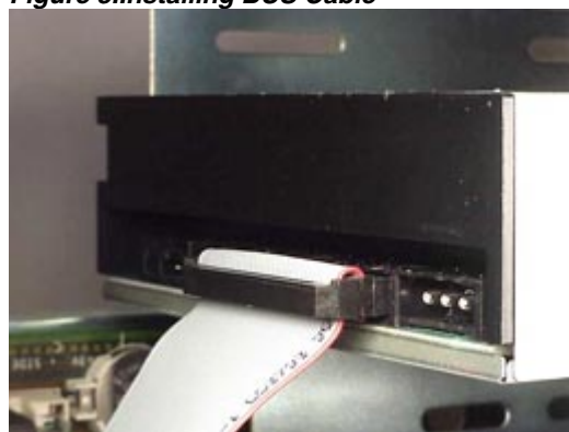
Figure 3. Installing BUS Cable
