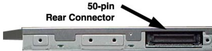
Figure 1. SD-R6012 DVD Writeable Drive Rear Panel – Connector
