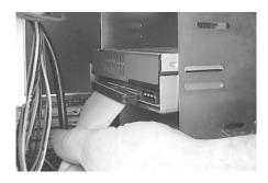
If you are replacing your SCSI CD-ROM: connect DVD-RAM to the SCSI interface connector that the CD-ROM was connected to. If DVD-RAM is an addition to a SCSI CD-ROM: daisy-chain the DVD-RAM with a custom built SCSI interface cable (not supplied with kit).
