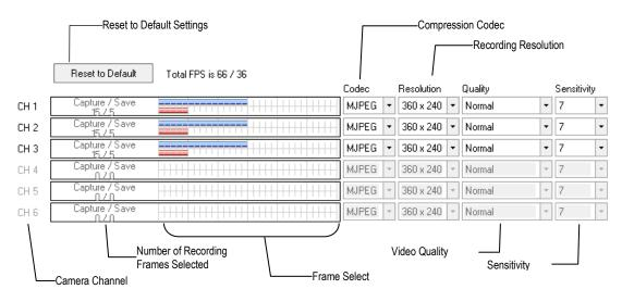
**Note** The red FPS record slider cannot exceed the blue FPS capture slider
