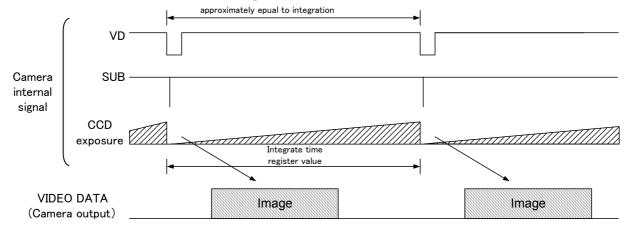
[Electronic shutter mode, Random trigger shutter mode, Exposure time: Register Value control]
