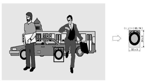
In the scalable mode, this camera reads out only the necessary portions at the standard speed while it scans through other unnecessary portions at high speed, so the trigger interval can be shorter if the vertical cutout width is small. However, the trigger interval cannot be short in the horizontal direction even if the cutout width is small due to the operation mechanism of the CCD sensor.
