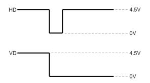
The amplitude level is the representative value when terminated with  $10k\Omega$ . Output is enabled when the rear panel HD/VD signal input/output switch is set to the INT side.
