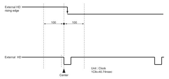
The phase relationship of the external HD and VD should correspond to the center phase (i.e., the external HD falling edge) as illustrated in the above diagram.
